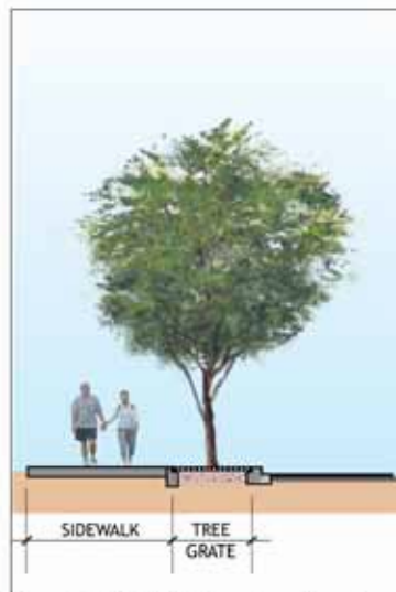
Figure 5.4.4.l: TYPE 2 - Sidewalk and trees in grates.
