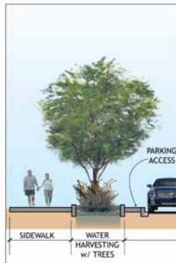
Figure 5.4.4.m: TYPE 3 - Sidewalk and water harvesting landscape with trees and paved parking access.
