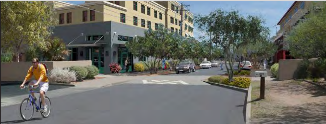
Figure 5.4.5.a: Simulation illustrating a chicane providing traffic calming and pedestrian amenities at an entry point between new development on Grant Road and an adjacent neighborhood.
