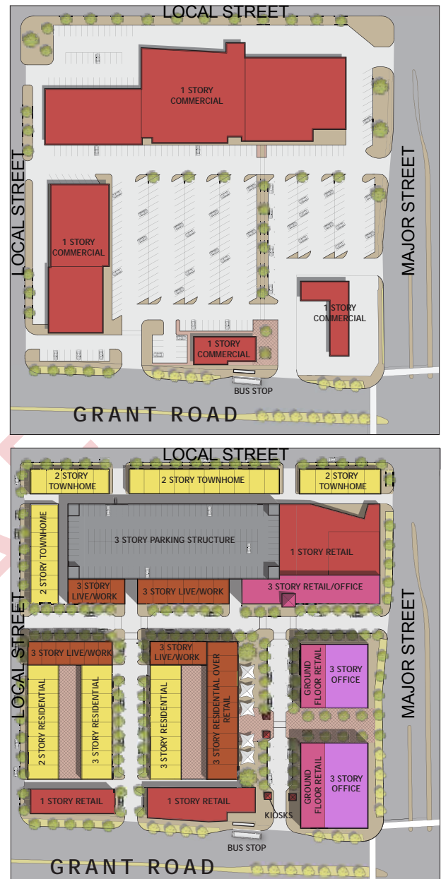
Figure 5.4.3.a: Diagrammatic plan of before and after showing how an existing shopping center might redevelop using the GRD, illustrating how new streets create blocks sized to meet the design standards.
