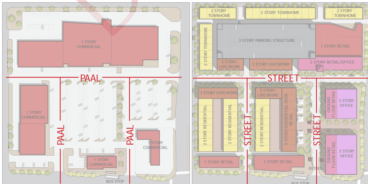
Figure 5.7.1.b.: Illustration showing the conversion of a main parking aisles and walkway connections into new streets within a shopping center redevelopment.
