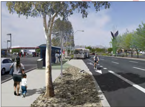
Figure 5.4.4.b and 5.4.4.c: Examples of buffering between the pedestrian realm and the roadway, a photo of a built example and a simulation of the Grant Road Improvements.
