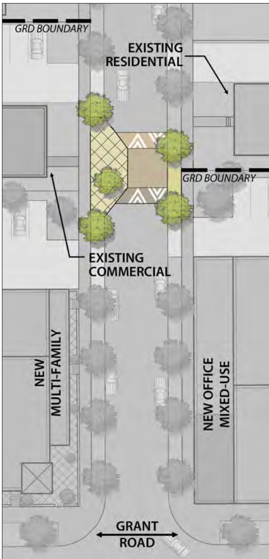
Figure 5.4.5.b: Diagram of a chicane located between driveways.
