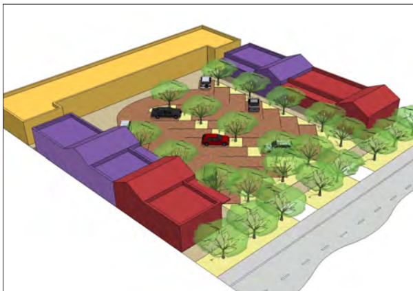
Figure 5.3.a: Horizontal Mixed Use Diagram showing non-residential uses at the street and residential uses at the rear.
