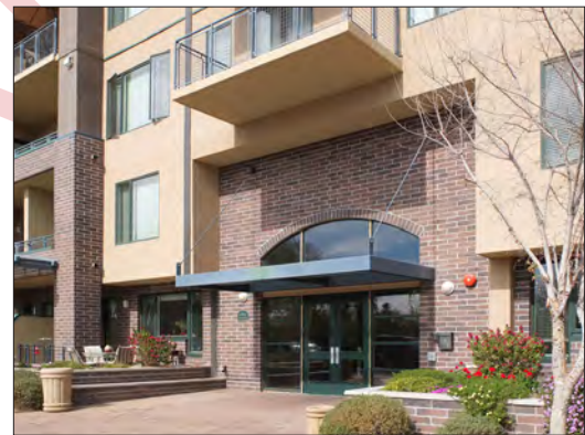
Figure 5.6.2.s: Photo example of a clearly defined building entrance. This lobby entry is distinguished from the individual unit entry to the left by its large-scale awning and the entry plaza.
