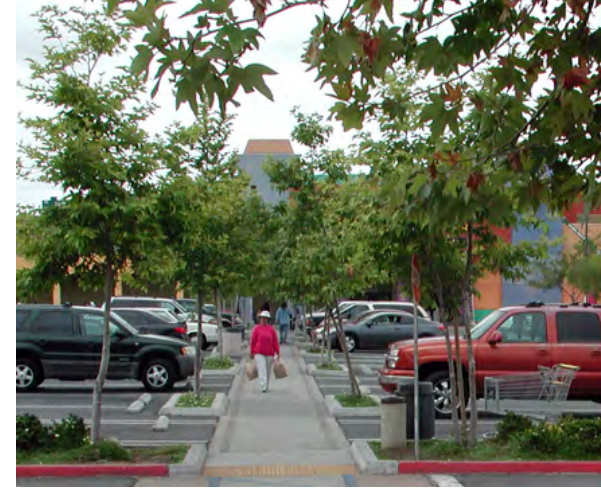
6’ wide walkways, clear of vehicle overhangs, parallel to parking aisles are required at a minimum spacing of every four rows.
